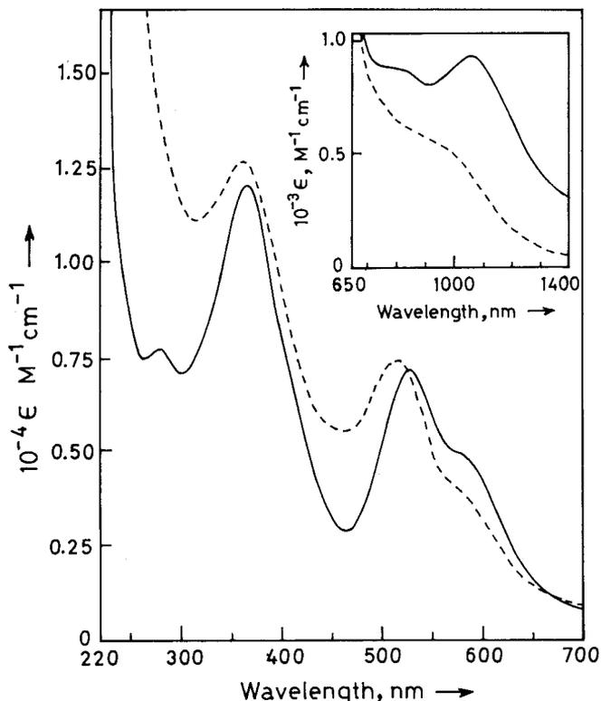
FIGURE 1 Electronic spectra of (a) *cis*-OsCl<sub>2</sub>(ClaaiMe)<sub>2</sub> (—) and (b) *trans*-OsCl<sub>2</sub>(ClaaiMe)<sub>2</sub> (----) in CH<sub>2</sub>Cl<sub>2</sub>.
