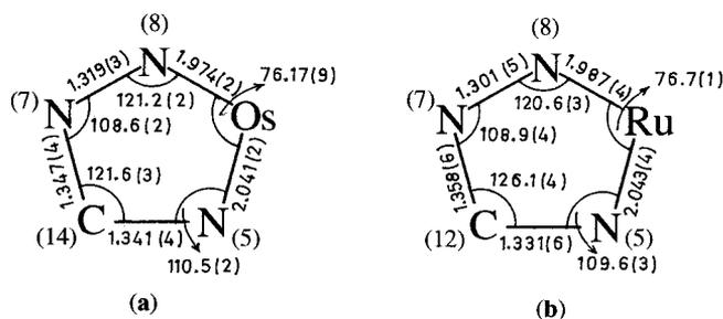
FIGURE 4 Dimensions of chelate rings with esd of (a)  $ctc\text{-OsCl}_2(\text{MeaaiMe})_2$  and (b)  $ctc\text{-RuCl}_2(\text{MeaaiMe})_2$ .
