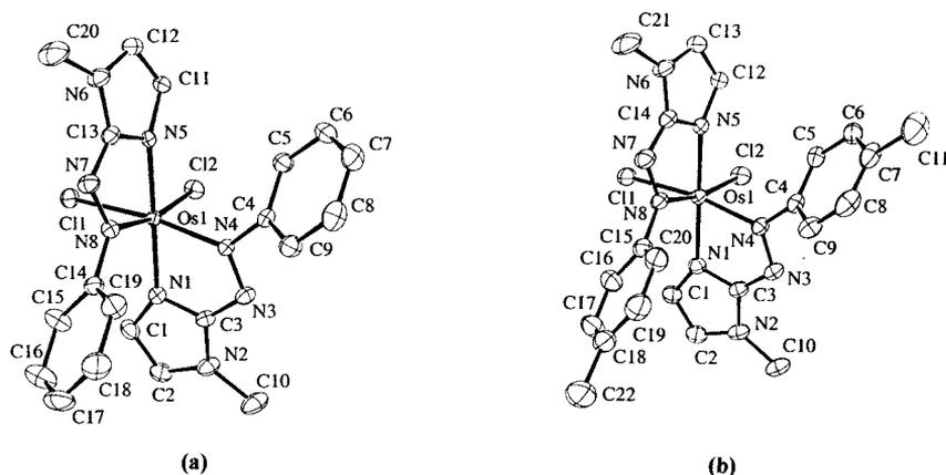
FIGURE 3 ORTEP plot and atom-labelling scheme for (a) *ctc*-OsCl<sub>2</sub>(HaaiMe)<sub>2</sub> and (b) *ctc*-OsCl<sub>2</sub>(HaaiMe)<sub>2</sub>.
