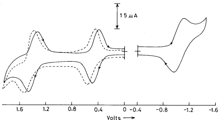
FIGURE 5 Cyclic voltammogram of *ctc*-OsCl<sub>2</sub>(ClaaiMe)<sub>2</sub> (—) and *ccc*-OsCl<sub>2</sub>(ClaaiMe)<sub>2</sub> (---) in MeCN using a Pt-disk milli electrode at 298 K, SCE reference and TBAP (0.1 M) supporting electrolyte.
