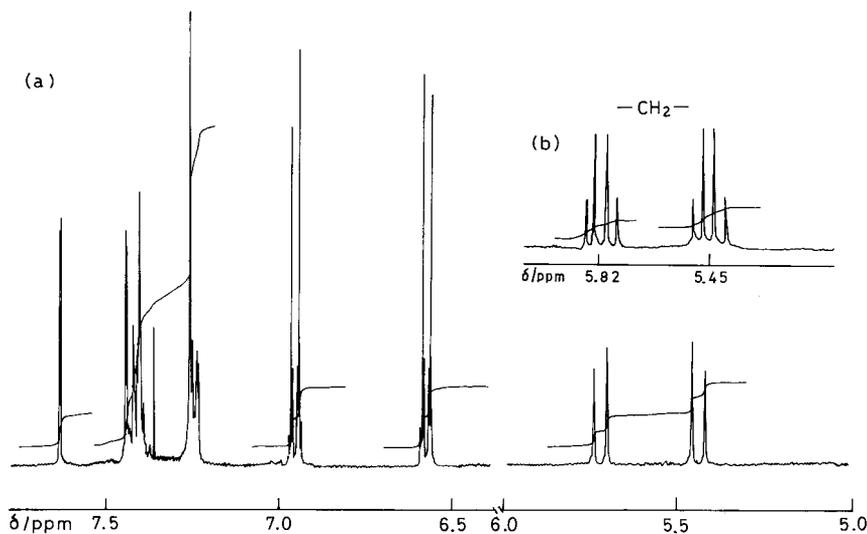
FIGURE 2  $^1\text{H}$  NMR spectra of (a) *ctc*- $\text{OsCl}_2(\text{ClaaiCH}_2\text{C}_6\text{H}_5)_2$  and (b)  $-\text{CH}_2-(\text{C}_6\text{H}_5)$  part of *ccc*- $\text{OsCl}_2(\text{ClaaiCH}_2\text{C}_6\text{H}_5)_2$  in  $\text{CDCl}_3$  at 298 K.
